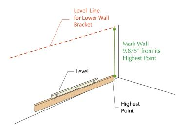
2. At the high point you determined on the floor, mark a level horizontal line on the wall that is 9.875" from the floor by snapping a chalk line, using a laser level or marking along the straight edge of a carpenter's level. If the floor is sloped you may need to make adjustments. This will establish the height on the wall where the lower mounting bracket will be installed.
